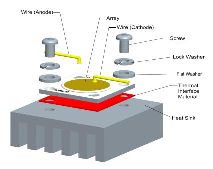
Cree recommends the following at all times when handling XLamp CM family LEDs or assemblies containing XLamp CM family LEDs:
