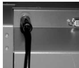
Screw-type power input
