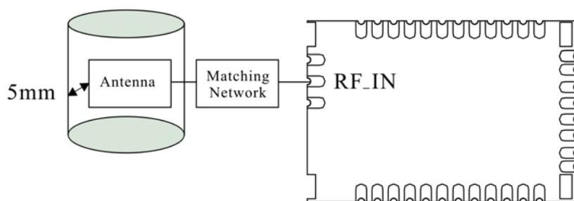
Figure 22: Leave 5mm Clearance Space from the Antenna
