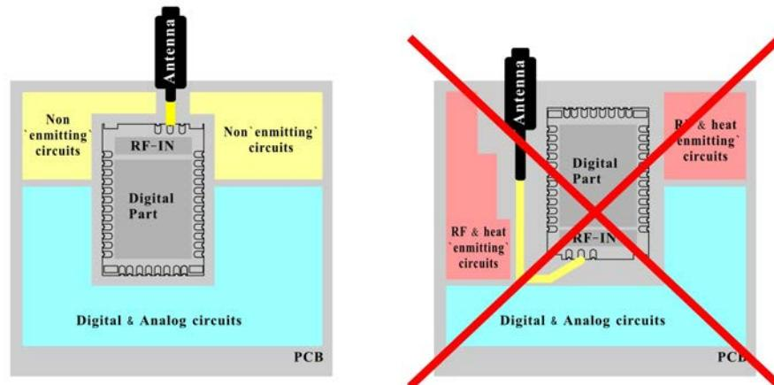
Figure 21: Placement the Module on a System Board
