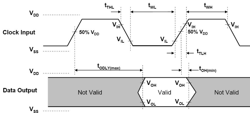
Figure 17: SDIO HS Output Timing
