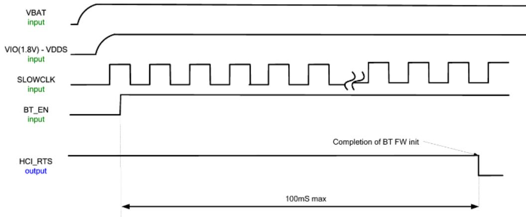
Figure 5: BT/BLE Power up Sequence
