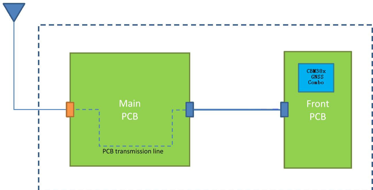
**Figure 12: GPS Signal routing inside a head unit**
