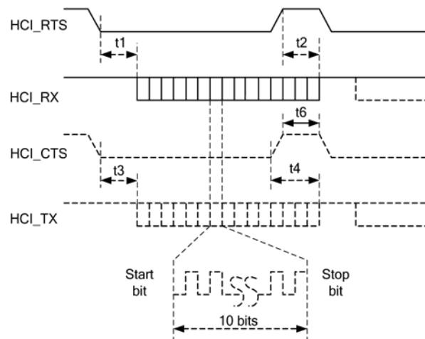
Figure 13: UART Timing Diagram
