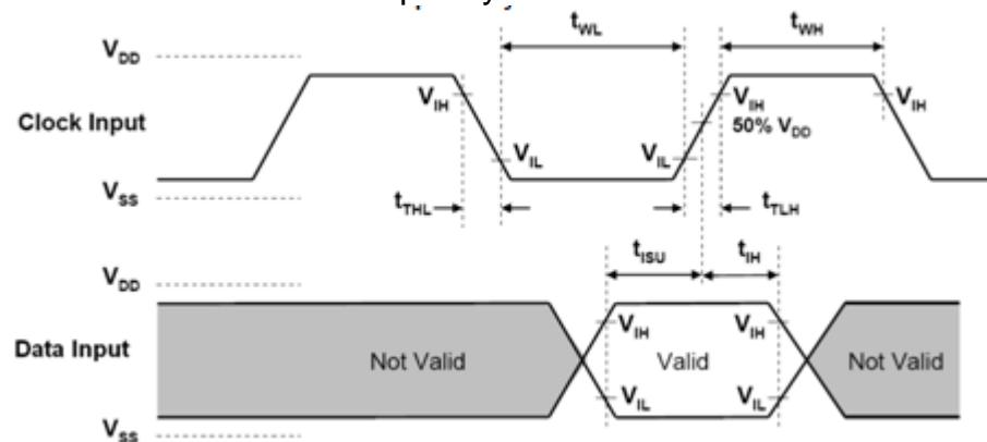
Figure 16: SDIO HS Input Timing
