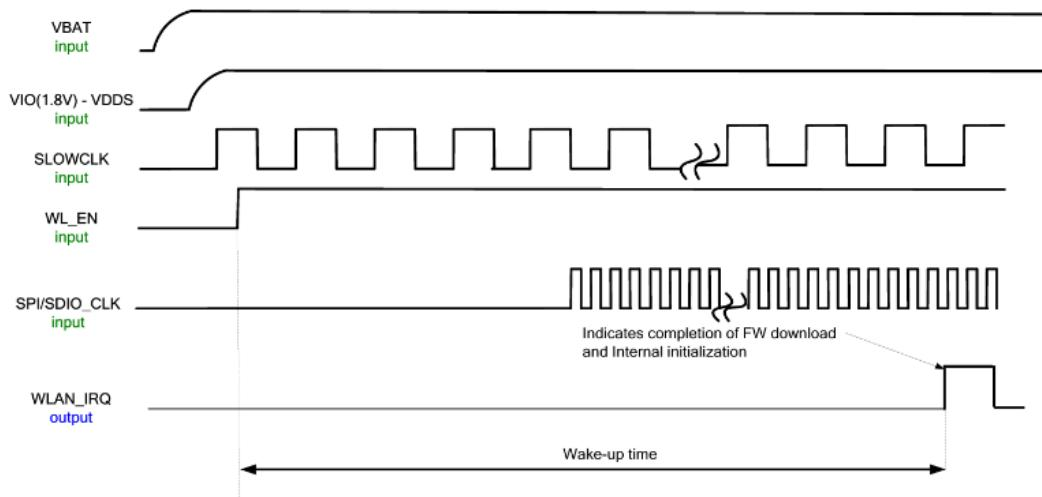
Figure 4: WLAN Power up Sequence
