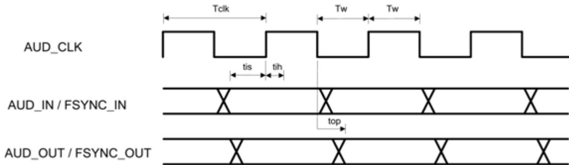
Figure 18: PCM Interface Timing
