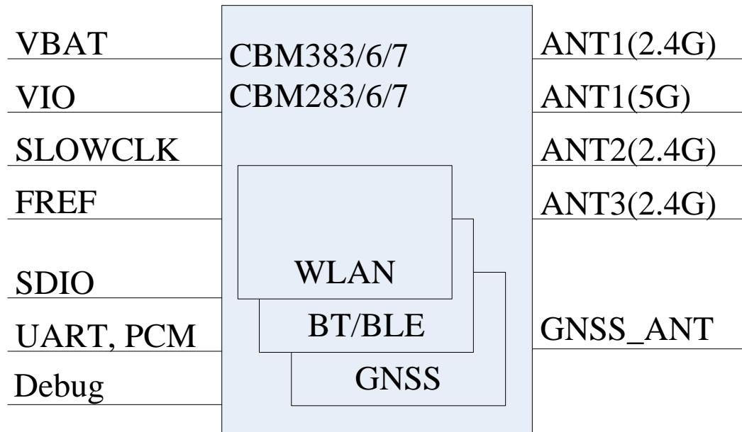
Figure 1: Block Diagram
