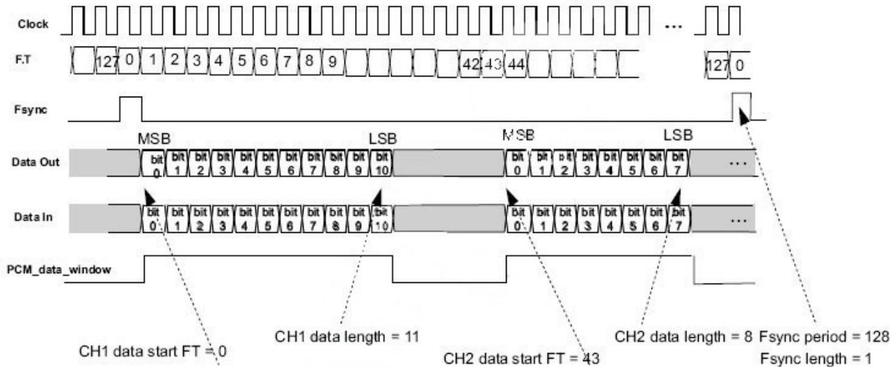
**Figure 7: 2 Channels PCM Bus Timing**
