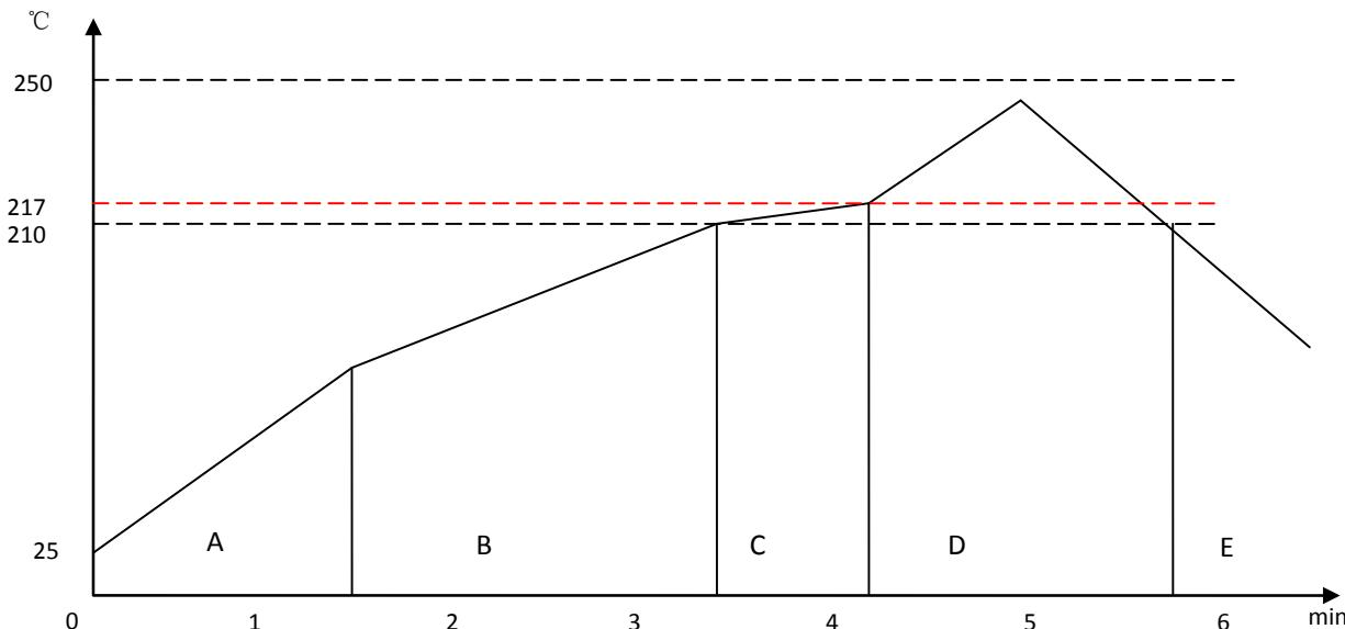
Figure 24: Recommended Reflow Profile
