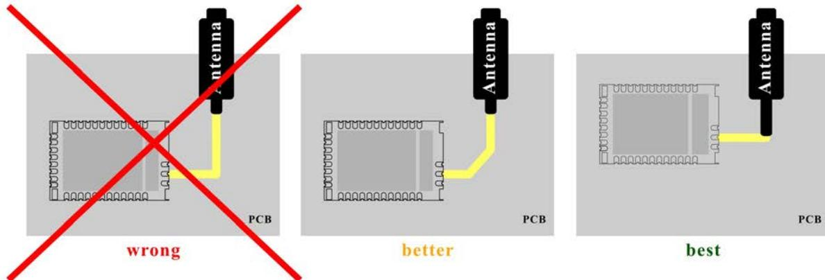
**Figure 23: Recommended Trace Connects Antenna and the Module**
