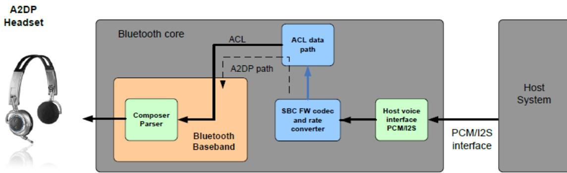
Figure 9: Device Assisted A2DP
