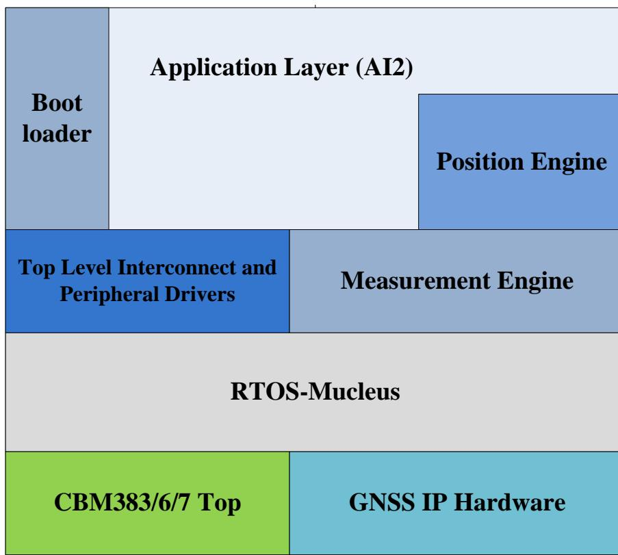
Figure 10: GNSS SW Architecture
