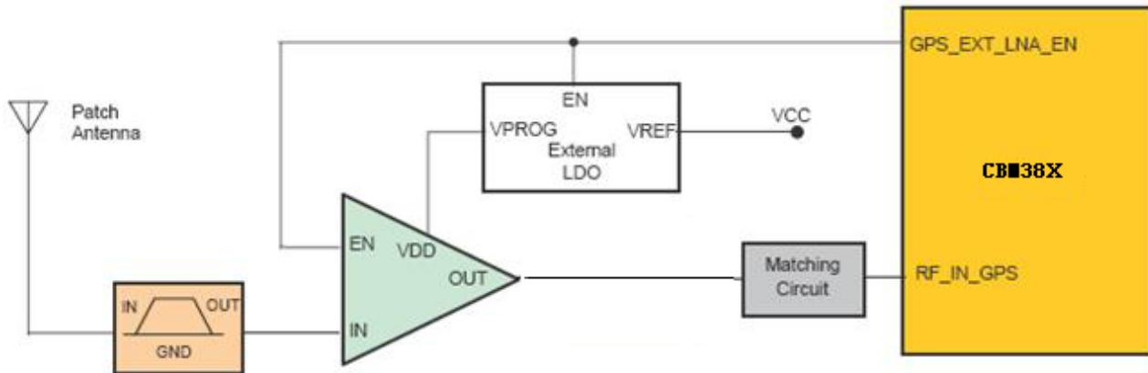
**Figure 11: External LNA Powered Using External LDO**
