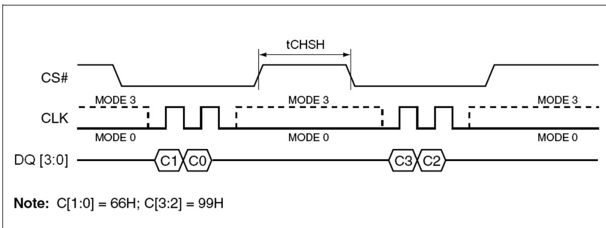
**Reset-Enable and Reset Sequence Diagram in QPI Mode**
