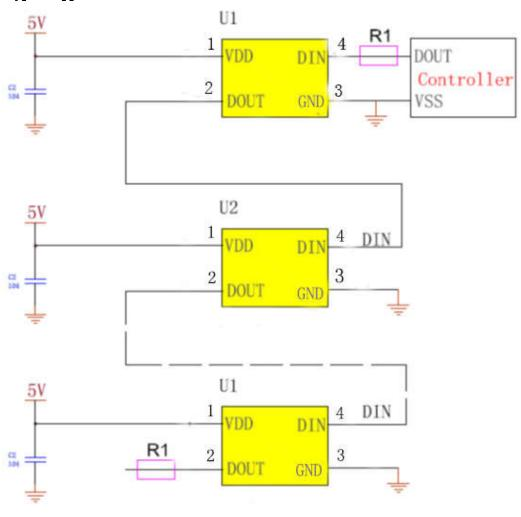
In the practical application circuit, the signal input and output pins of the IC signal input and output pins should be connected to the signal input and output terminals. In addition, in order to make the IC chip is more stable, even the capacitance between beads is essential back;
