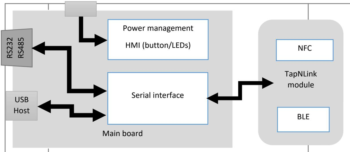
The TapNPass embeds a standard TapNLink module. This module manages radio communication, while serial communication is performed by the main board.
