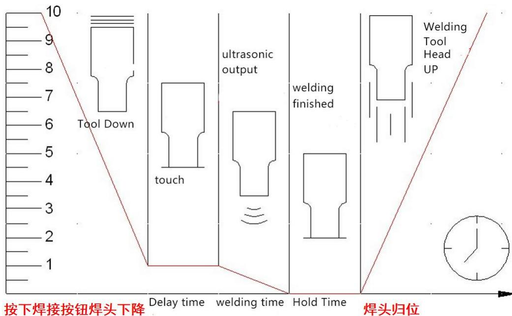
**Delay time:** the time from pressing the welding button to pressing the welding part. That is, the time of phase 1 to phase 2 in the figure, which will be related to the cylinder travel and falling speed. If I do not know how much to set, set a relatively large value, and then reduce it according to the circumstances, such as 0.8s is good. Can be set up 0 ~ 9.99 s
