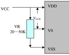
We recommend allowing field adjustment of V0 for all designs. The optimal value for V0 will change with temperature, variations in VDD, and viewing angle. V0 will also vary module-to-module and batch-to-batch due to normal manufacturing variations.
