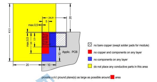
Figure 6: FSC-BT836B Restricted Area
