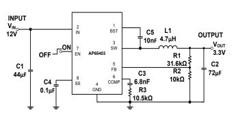
Figure 1. Typical Application Circuit
