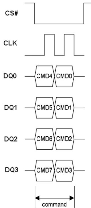
**Figure 31.1 Chip Erase Sequence in QPI Mode**
