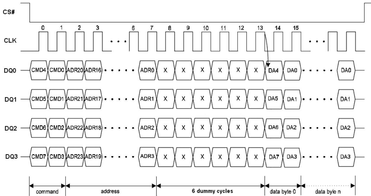
**Figure 17.1 Fast Read Instruction Sequence in QPI Mode**
