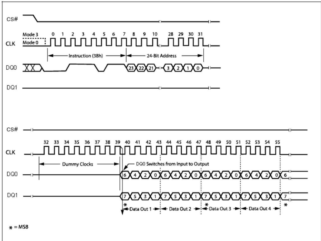
**Figure 18. Dual Output Fast Read Instruction Sequence Diagram**
