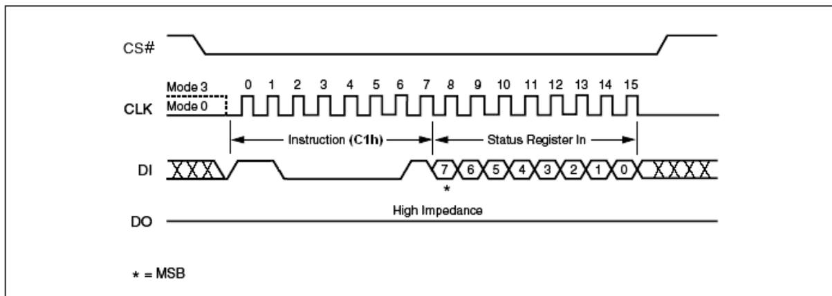
**Figure 15. Write Status Register 4 Instruction Sequence Diagram**
