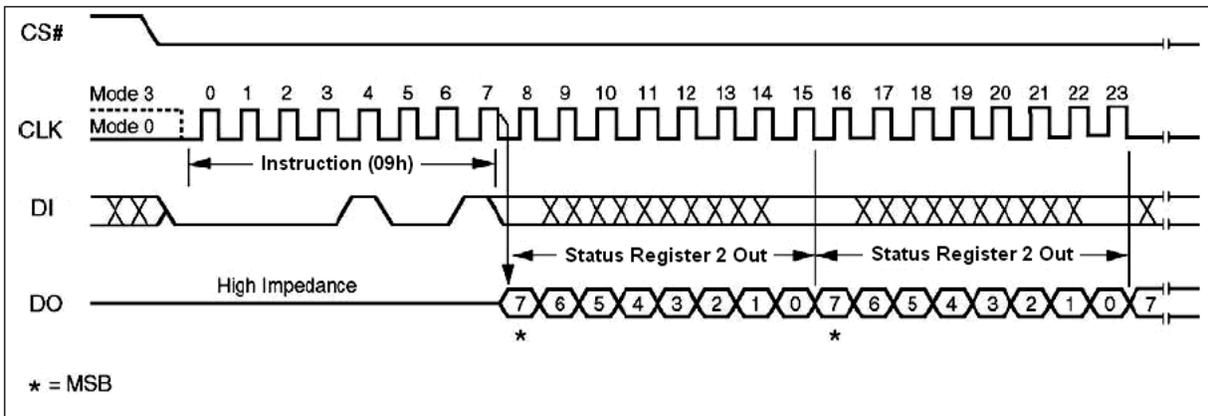
**Figure 12. Read Status Register 2 Instruction Sequence Diagram**
