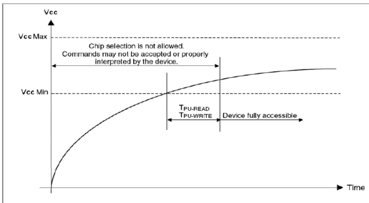
**Figure 39. Power-up Timing**
