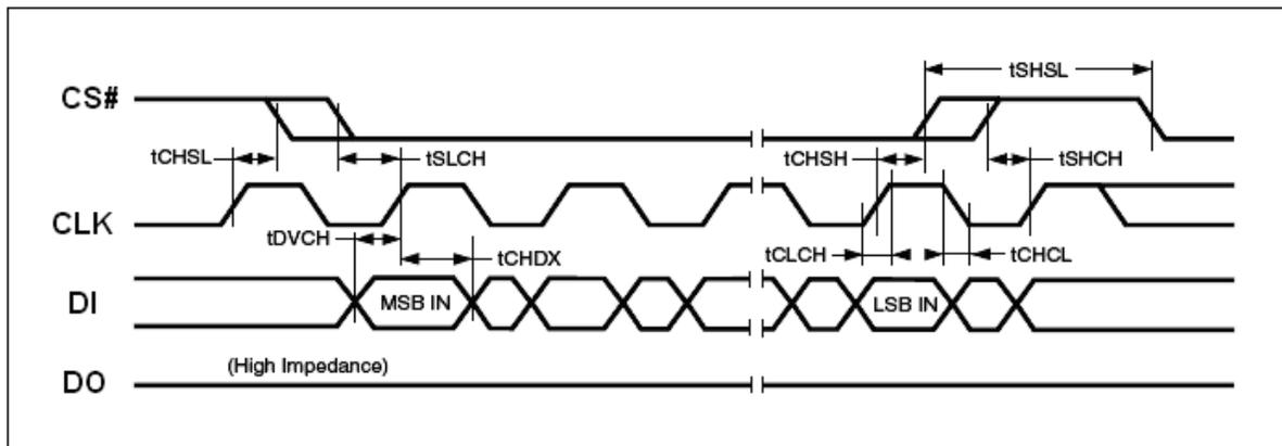
**Figure 42. Input Timing**
