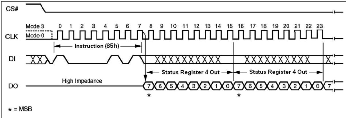
**Figure 13. Read Status Register 4 Instruction Sequence Diagram**
