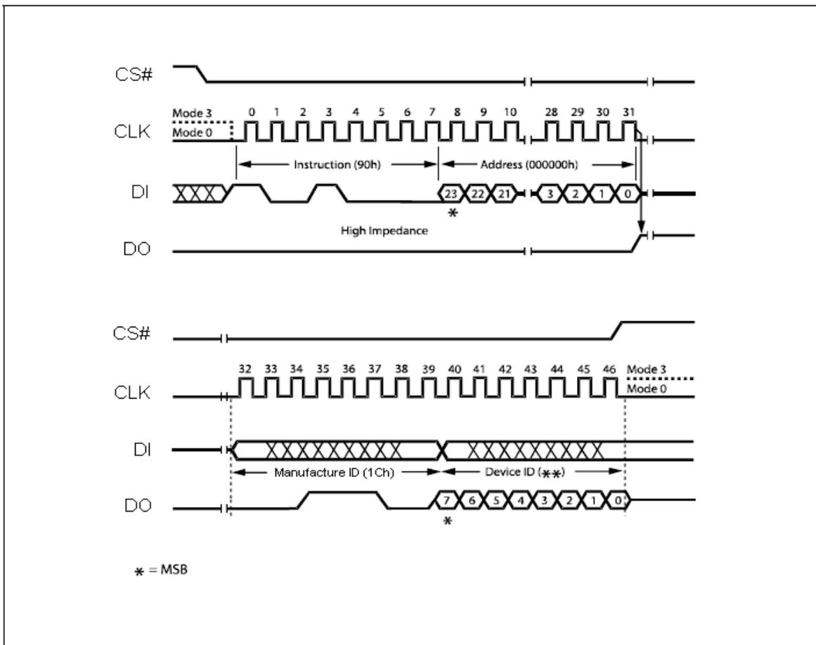
**Figure 35. Read Manufacturer / Device ID Diagram**
