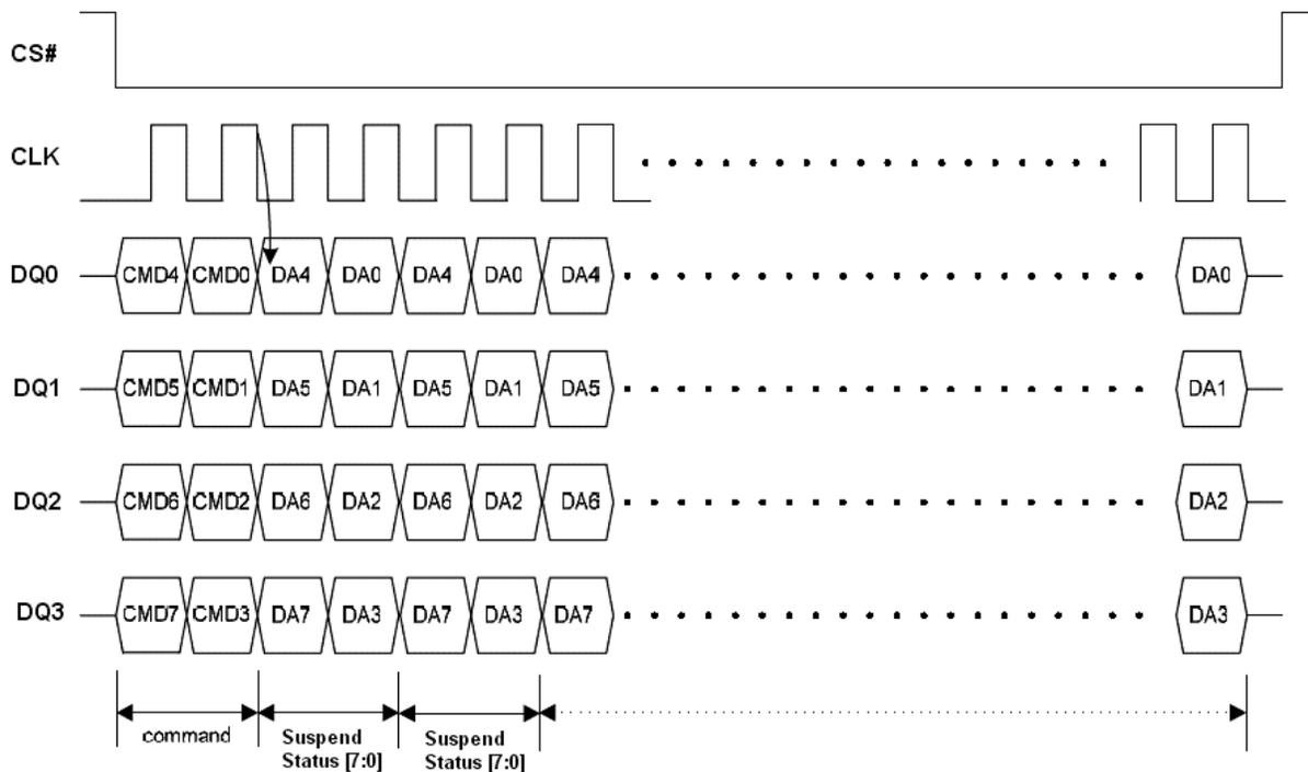
**Figure 13.1 Read Status Register 4 Instruction Sequence in QPI Mode**
