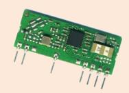
Wide supply voltage range from 2.1 to 5.5 Vdc.
