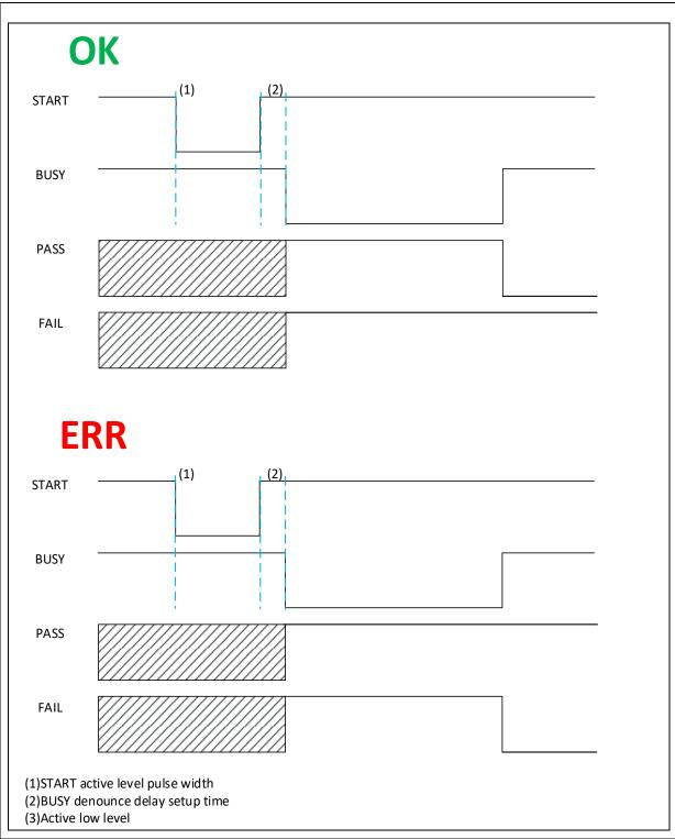
Figure 26. Typical timing diagram of machine programming control
