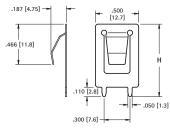
MATERIAL: .012 (.30) Spring Steel, Nickel Plate
