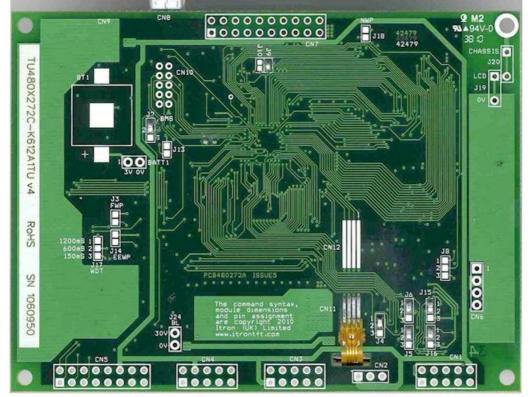
Rear View TU480X272C-K612A1TUv5 with factory jumper setting.
