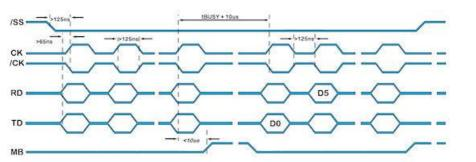
SPI Synchronous Serial Communication
