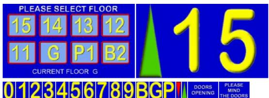
The user can select a floor and travel from any floor to another floor. The arrow is selected according to direction. Warning signs for doors opening and closing are used. Variables are used to store the current floor and destination floor. An RS232 interface could be added to communicate with other floor indicators. Download Image Files <a></a></a>
