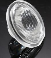
Family Eva Lens Type LED MC-E Color Clear Diameter 35 mm Height 16.4 mm
