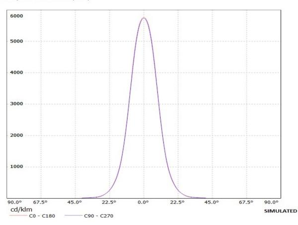
Luminaire: Ledil Oy FA10678\_CMC-SS FA10678\_CMC-SS Lamps: 1 x CREE MC-E (white)
