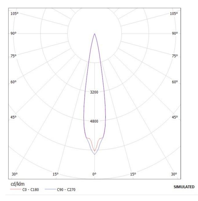
Luminaire: Ledil Oy FA10677\_CMC-D FA10677\_CMC-D Lamps: 1 x CREE MC-E (white)
