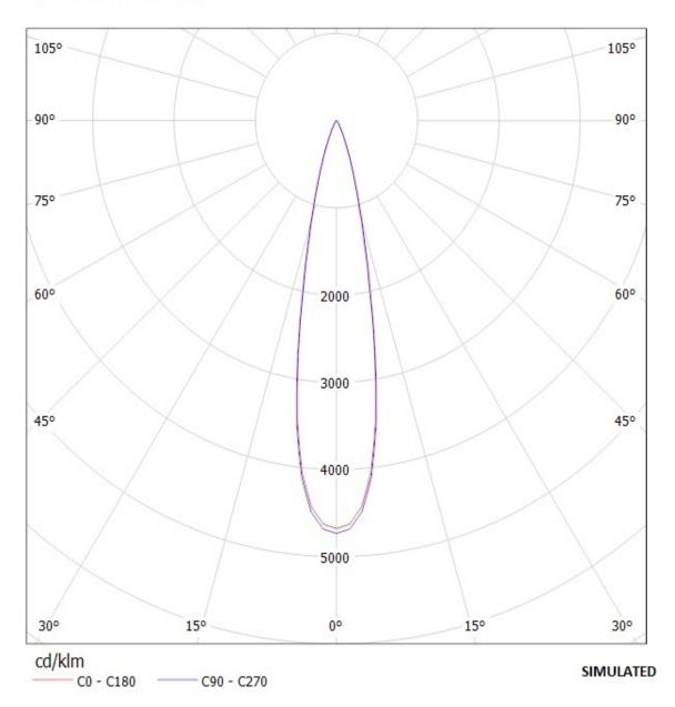
Luminaire: Ledil Oy FA10676\_CMC-M FA10676\_CMC-M Lamps: 1 x CREE MC-E (white)
