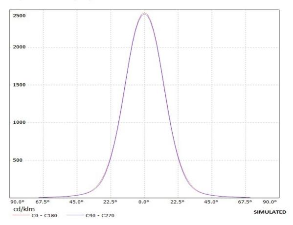
Luminaire: Ledil Oy FA10676\_CMC-M FA10676\_CMC-M Lamps: 1 x CREE MC-E (white)
