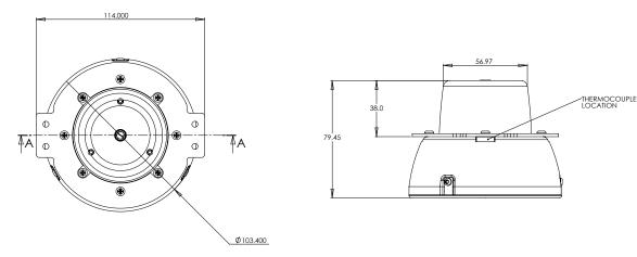
Operating temperature of the Cree LED Module LMR4 is between 0 °C and 50 °C. The lifetime and performance estimates described in this document apply only if the product's Thermal Management Guidelines (below) are adhered to and no modifications are made except as described in this document.
