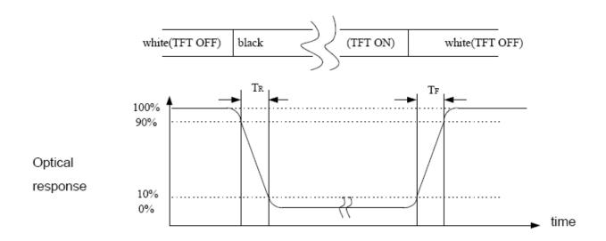
Note (4) Definition of optical measurement setup
