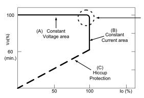
Typical LED power supply I-V curve
