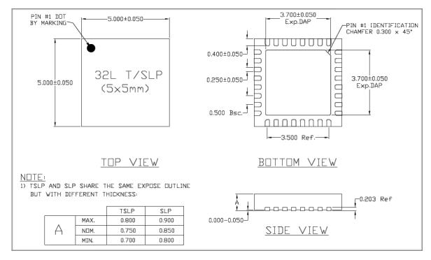
Figure 6-1. ESP8266EX Package
