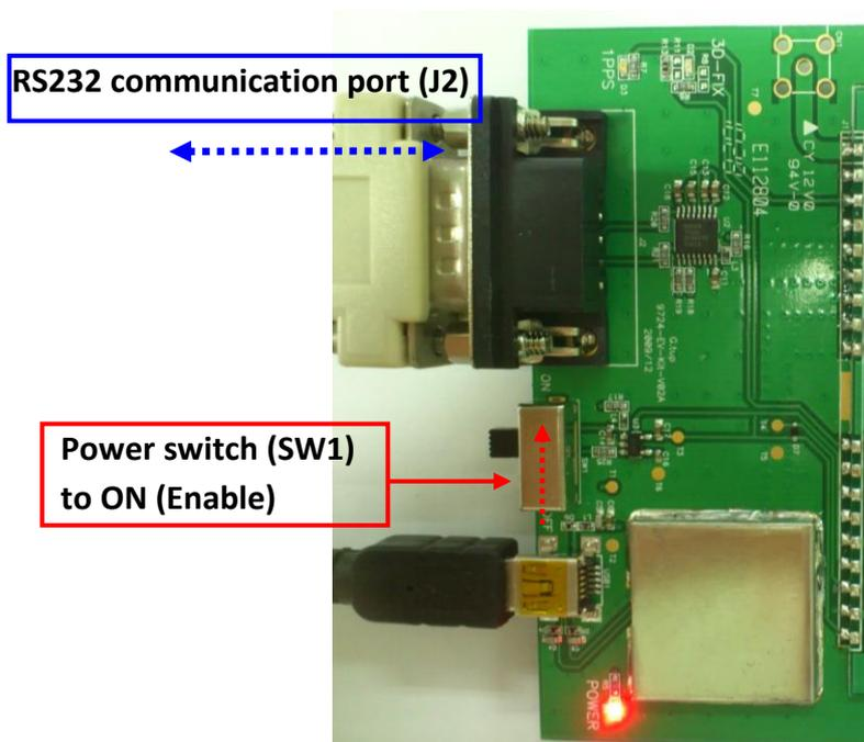
GNSS Simulator Hardware set up as below:
