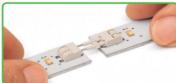
Assembly: Place PCB on a flat surface and insert links into terminal blocks on adjoining PCBs.
