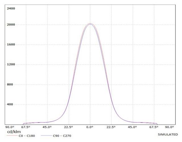
Luminaire: Ledil Oy 10446\_Cute-4-SS 10446\_Cute-4-SS Lamps: 1 x Cree XR-E 4PCB (white)
