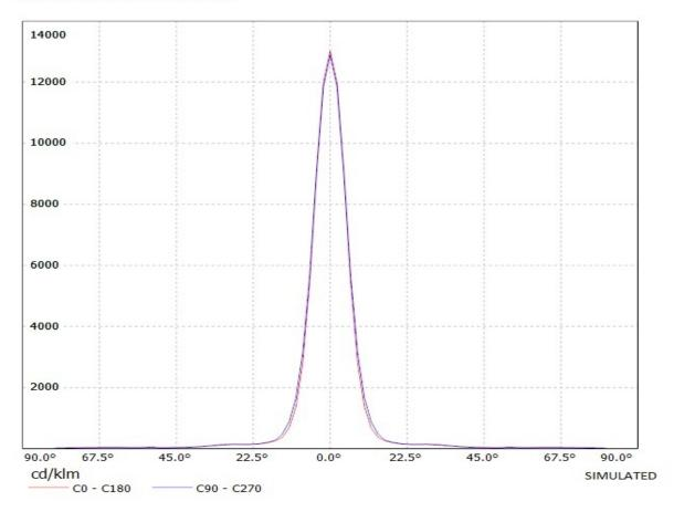
Luminaire: Ledil Oy 10446\_Cute-4-SS 10446\_Cute-4-SS Lamps: 1 x Cree XR-E 4PCB (white)
