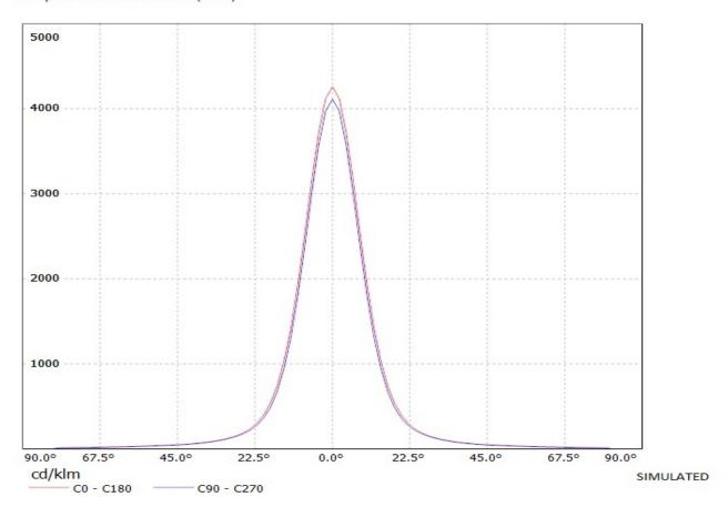
Luminaire: Ledil Oy 10447\_Cute-4-M 10447\_Cute-4-M Lamps: 1 x Cree XR-E 4PCB (white)
