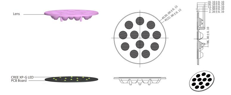
2. View assembly lens with MCPCB:
