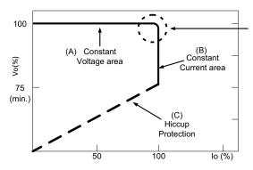
Typical LED power supply I-V curve
